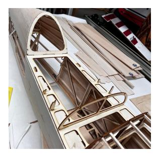
The Cockpit frame can now be assembled on the model, We recommend using greese proof paper, so it does now stick to the model.
