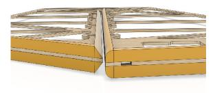
The Front of the Elevator is to have a 45% chamfer to each side. This will give you 45 Degrees Of Movement, Please Adjust to your Flying Style, But we do not recommend more than 50 Degrees or less than 30 Degrees. as this is a very sensative surface.
