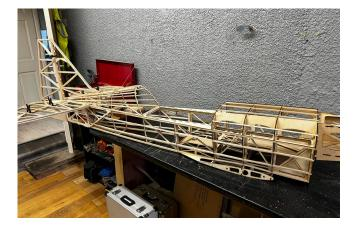
Assemble the engine box using epoxy., Make sure the engine box has right hand thrust (Like the shown photo)
