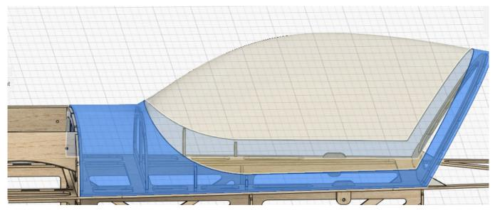
The Cockpit frame is sheeted as shown in the image. Use 2.4mm Balsa
