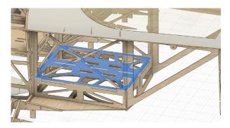
Now we can gain access from above, we can now add the servo tray. Use epoxy on all mounting surfaces.
