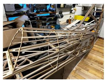
After the elevators are mounted correcly, The 5mm x 5mm Stringer can now be added to the rear turtle deck! Superglue is fine for this.
