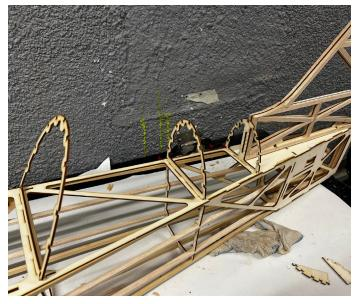
FT2, F3T AND F4T Can be glued in place Using epoxy. You can also at this point add TWM
