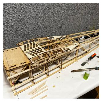
Fit The 6.5 mm x 9.5mm Balsa wood Stringers to the Fuselage. You will need to join these with a scarf joint. Use Superglue to a good strong bond. Ensure these run in to the Rear UC Sides. We recommend adding a joining strip inside the rear UC area,
