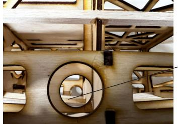
The Phenolic tube can be added to the model. You will need to notch the Obechi Middle Strip to get the -Phenolic in place. Glue in place with Epoxy.
