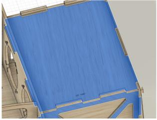
Once the fuselage is dried, you now need to add the undercarriage Side doubler, Undercarriage Doubler and Main UC Plate. Use 30 Minute Epoxy,
