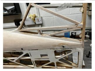
on F4 and F2 you now need to add the steel work for the wings, these are in the Ali Pack supplied with the Kit. ON F4 AND F2 the ali fits in the same place. as shown on drawing,
