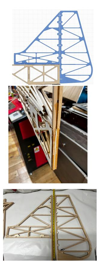
Construction is similar to elevator using the same 6.5mm x 9.5mm Spruce and 6.5mm x 9.5mm Balsa. inished thickness is 22mm
