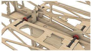
In the Kit, there is also 4 Parts Called STM. These parts are used to set the Elevator Angles
