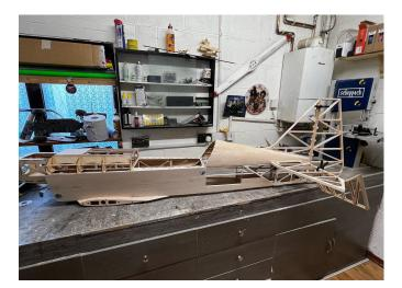
There are also a few other areas at the bottom of the model that will need sheeting to make things neat for covering and Rudder Control Wire Exits.
