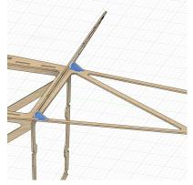
Rear Turtle Deck Ribs can also be added, use CA to get the angle of F6T Correct. These Can be glues with Superglue. Do Not Place F9T in Place Just yet
