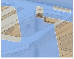
Leave F1 Hanging over the edge of the deck and now add all other fuselage ribs \* F6 - F8 - Ensure these are square to fuselage, use super glue to stick in place.
