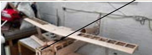
Once complete, Add the final few 3.2mm x 3.2mm Balsa Stringers with superglue, and sheet the top section of the model.
