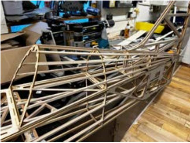
After the elevators are mounted correctly, The 3.2mm x 3.2mm Stringer can now be added to the rear turtle deck! Superglue is fine for this.
