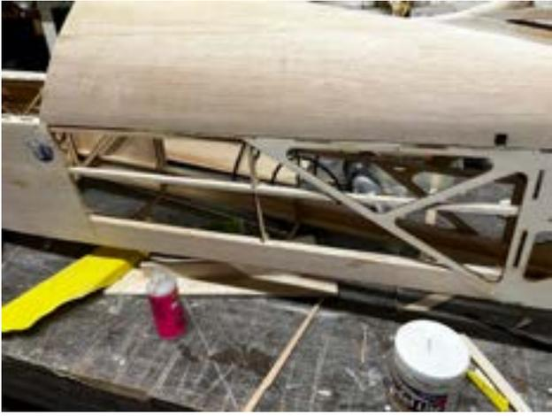
There are also a few other areas at the bottom of the model that will need sheeting to make things neat for covering and Rudder Control Wire Exits.
