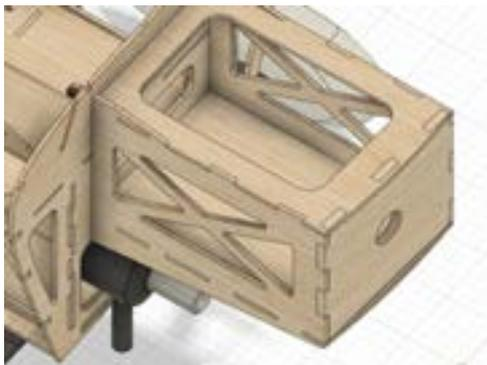
Assemble the engine box using epoxy., Make sure the engine box has right hand thrust ( Like the shown photo)
