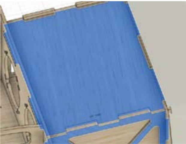
Image Shows Undercarriage Doubler which fits on the inside of the model
