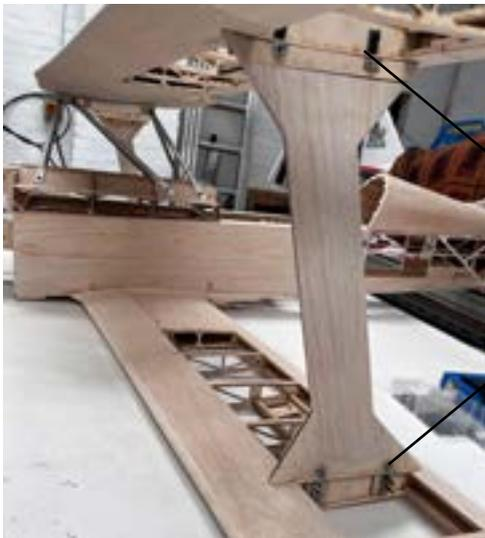
The Interplain Struts are fully sheeted on one side with 3mm Balsa.
