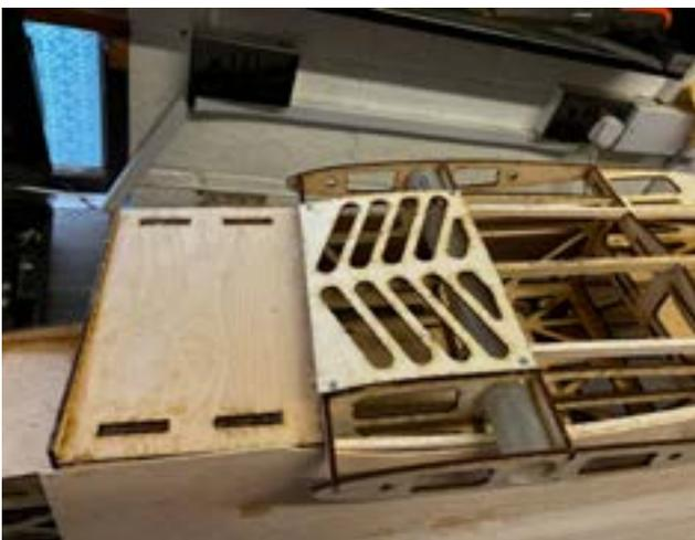
The Exhaust Hatch can now be added to the model by using scrap pieces of wood for screw points in each corner.
