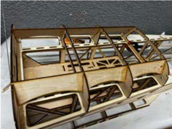
FT2, F3T AND F4T Can be glued in place Using epoxy.
