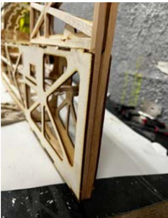
The Rudder Stab Can be added to the fuselage. This interlocks in to F8T.
