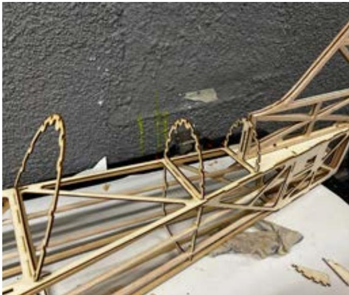
Rear Turtle Deck Ribs can also be added, use CA to get the angle of F6T Correct. These Can be glued with Superglue. Do Not Place F9T in Place Just yet
