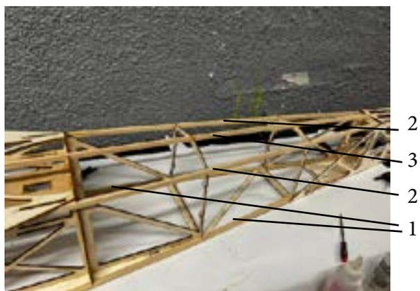
Please ensure no3 Runs under the Rear UC Plate and is glued with epoxy. Make sure to get a Hard fit against Rear UC Sides and Rear UC Plate.
