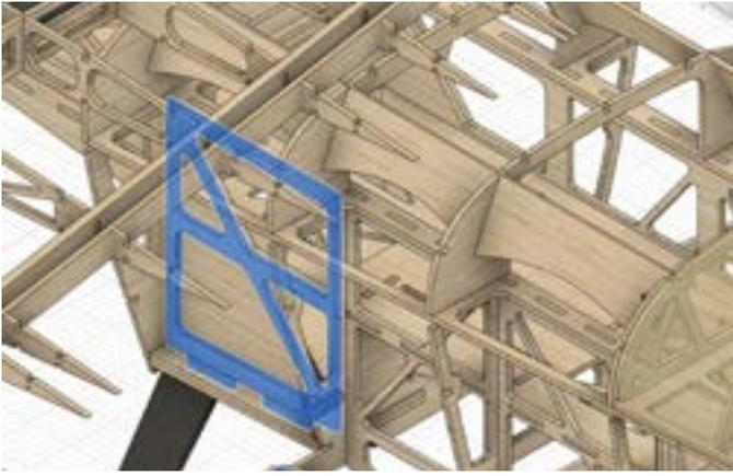
Once the fuselage is dried, you now need to add the undercarriage Side doubler, Undercarriage Doubler and Main UC Plate. Use 30 Minute Epoxy,
