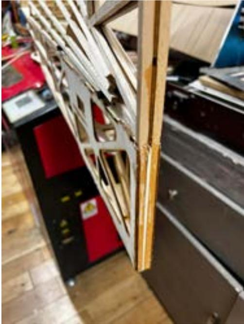
A small Strip of balsa wood can be glued between the spruce on the stabs. Superglue will be perfect for this.
