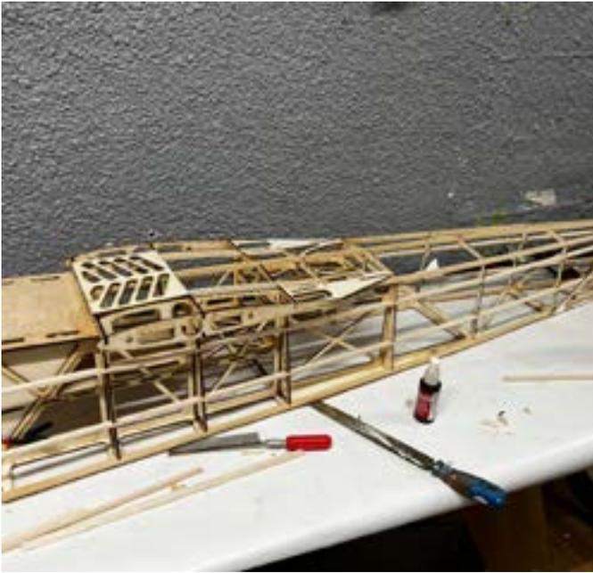
Fit The 6.5mm x 3.2mm Balsa wood Stringers to the Fuselage.
