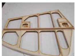
It is worth at this point trial fitting a servo of the type you are going to fit. Making mods to fit at this point will save you time later. ALSO AT THIS POINT YOU NEED TO HAND THE REAR STABS ie RH and LH. Please give consideration to cable runs of servos.
