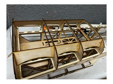
FT2, F3T AND F4T Can be glued in place Using epoxy. You can also at this point add TWM
