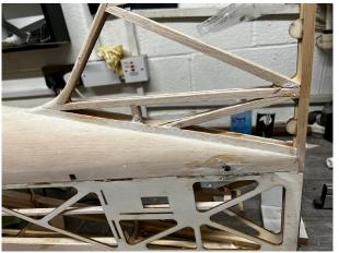
Ensure you cut the balsa around the rear Elevator Carbon Rods.
