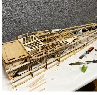
The Exhaust Hatch can now be added to the model by using scrap pieces of wood for screw points in each corner
