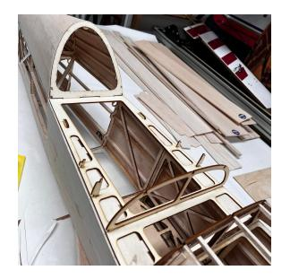
The Cockpit frame can now be assembled on the model, We recommend using greese proof paper, so it does now stick to the model.
