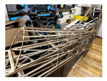
After the elevators are mounted correcly, The 4mm x 4mm Stringer can now be added to the rear turtle deck! Superglue is fine for this.
