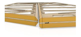
The Front of the Elevator is to have a 45% chamfer to each side. This will give you 45 Degrees Of Movement, Please Adjust to your Flying Style, But we do not recommend more than 50 Degrees or less than 30 Degrees. as this is a very sensative surface.
