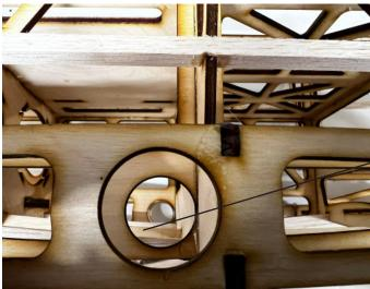
The Phenolic tube can be added to the model. You will need to notch the Obechi Middle Strip to get the Phenolic in place.
