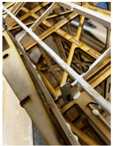
on F4 and F2 you now need to add the steel work for the wings, these are in the Ali Pack supplied with the Kit. ON F4 AND F2 the ali fits in the same place. as shown on drawing,
